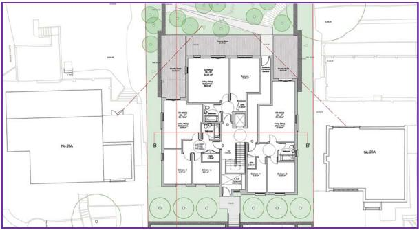
Image 8.4: 45-Degree Test on plan.
