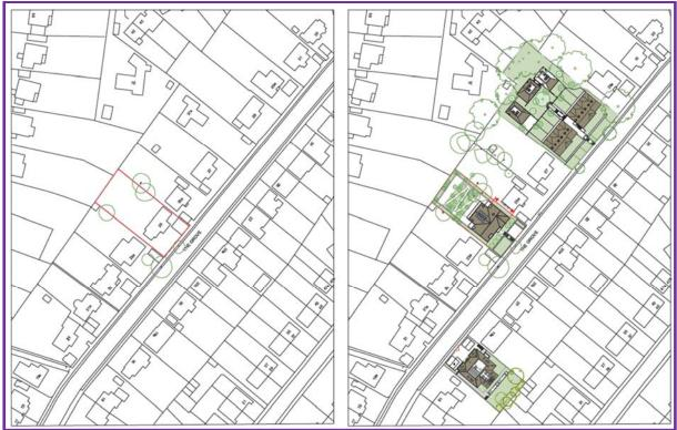
Image 8.1: Existing (Left) and Proposed Block Plans.
